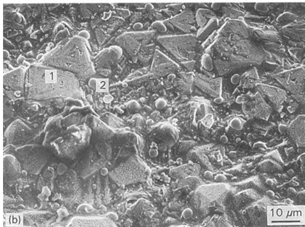
Figure 4 Scanning electron micrograph showing the surface morphology of laser-treated sample LT1: (a) overall morphology, (b) fine structure.
